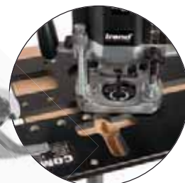
Bolt Recess Routed
