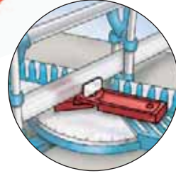
Position the long part parallel to the workpiece and set the sawblade parallel to the metal flag.
