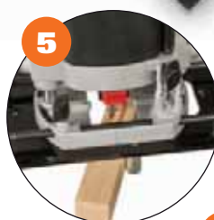
5 Offset Mortising For timber thickness 50mm to 200mm.
