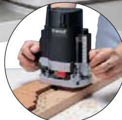
Template Guide Bush Routing
