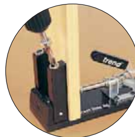
3. Drill pocket hole sockets
