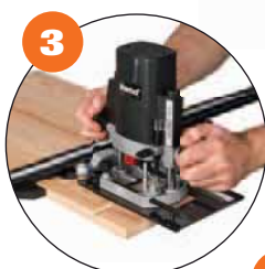
3 Clamp Guide Adjustable Grooving With 40mm micro adjustment.
