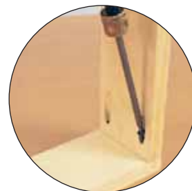
4. Drive self tapping screws to secure
