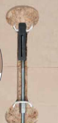
Joint Biscuit Jointed for Additional Strength
