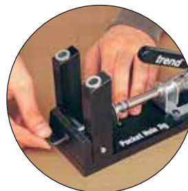
1. Adjust column position
