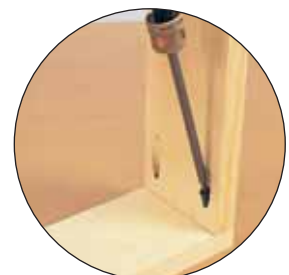
4. Drive self tapping screws to secure
