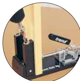
3. Drill pocket hole sockets
