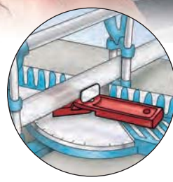
Position the long part parallel to the workpiece and set the sawblade parallel to the metal flag.
