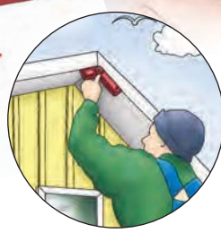
Position the tool in the unknown angle and the metal flag automatically halves the angle.
