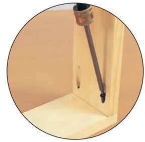
4. Drive self tapping screws to secure
