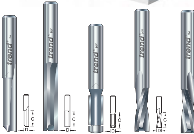
Refs. ACRS2/60 , ACRS2/6 & ACR2/80 Single flute for fast cutting.
