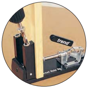
3. Drill pocket hole sockets
