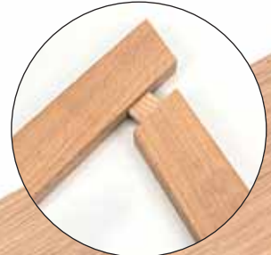
Angled mortises are constructed simply by cutting the shoulder of one component to the relevant angle.
