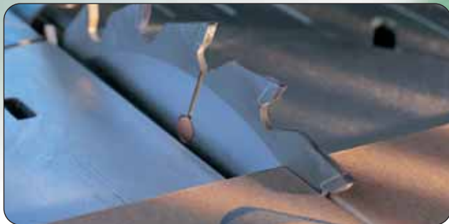
Alternate top bevel tooth form
