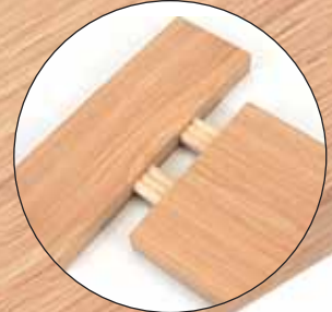
By using two or more loose tenons in line, wide components can be jointed, e.g. the middle rail of an internal door.
