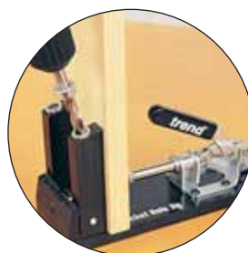
3. Drill pocket hole sockets.
