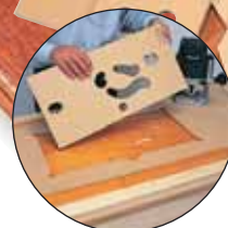
3. Reposition template and rout again.
