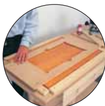
1. Clamp template frame to component.
