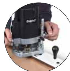
Rout Hinge Recess
