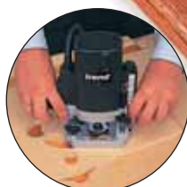
2. Position template and follow the slots using the special cutter.
