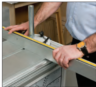
Fit the tenoning fence.
