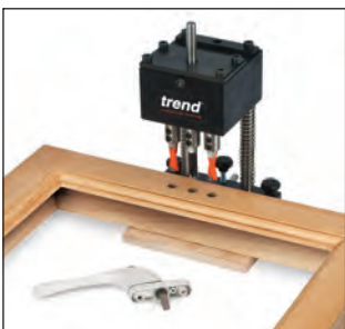
Drill the three holes for the Espagnolette handle. See page 59.
