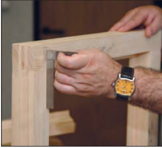
Dry assemble and check each joint.
