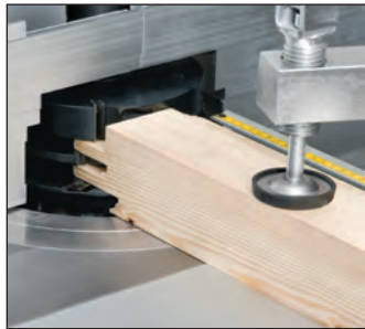
Slot and tenon the ends of each timber section of the outer frame and sashes. Always butt the timber sections against the back-fence. No stops are required. Repeat as necessary for each operation.
