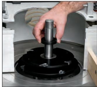
All spacers also have an identification number as they are part of the system.
