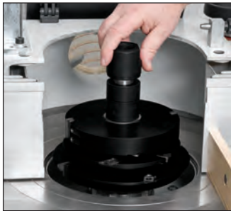
Fit the top spacer, followed by the nut and tighten it.
