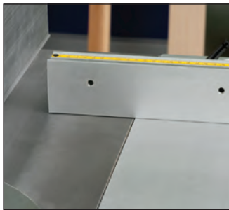
The tenoning fence on the Trend Spindle Moulder is pre-drilled with two M8 threads to take a wooden spluch block. See jig on page 57.
