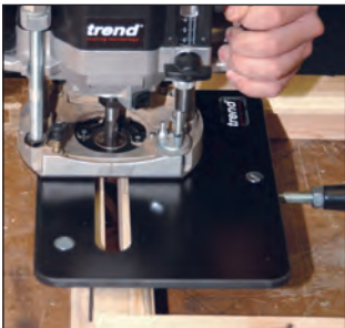
Rout the groove for the trickle vents, with the Trend Trickle Vent jig (see page 57).
