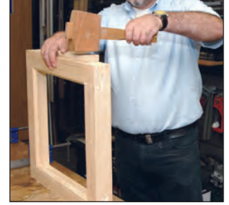
Lightly hammer each joint to ensure they are tight.
