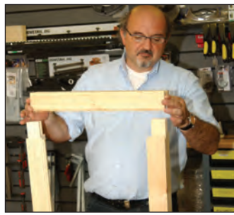
Glue up, assemble and clamp the sashes, and leave to dry. See top of page 8.
