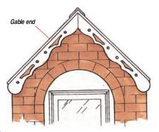
Replacing decorative timber barge boards requires repetitive machining of long boards to a set pattern. This therefore lends itself to routing operations using a template and a guide bush fitted to the router.
