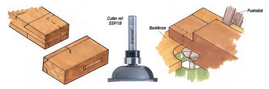
The shoulder scribe joint between mortise and tenon of a profiled frame requires special tooling.
