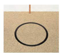
4. Unscrew the jig from the waste piece. Insert a spacer ring (three are supplied with each jig) into the hole. Invert the waste piece and fit it into the insert ring.
