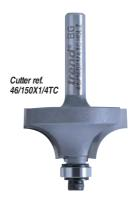
2. A bull-nose moulding will be required on three of the edges. For 1" (25.4mm) thick board, use a 1/2" (12.7mm) radius rounding-over cutter, Trend ref. 46/150X1/4TC or similar. Adjust the height of the cutter so that the top quirk is just clear of the top surface. The roller bearing fitted to the end of the cutter acts as the guide and runs along the centre of the board edge.
