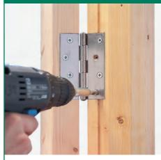
The Trend Snappy quick release drill system includes drill bit guides for quick drilling of fittings for hinges, drawer runners and other ironmongery pre-drilled with countersunk holes.
