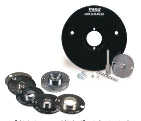
Guide bushes are available in different diameters to allow various diameter cutters to be accommodated. Many makes of router do not offer a range of guide bush sizes. Therefore a sub-base should be fitted to the base into which the full range of guide bushes can be fitted. These are available in diameters of 10mm to 32 in 2mm increments and also in 11, 17 and 40mm size.
