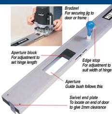
This is a portable template jig designed for recessing hinges in wooden doors and frames. The apertures and edge stops are initially set and the template is then ready for accurate recessing of the frame and the door without adjusting the jig.
