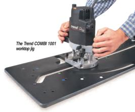
The jig consists of precision machined slots which guide the router. Bushes are positioned in various combinations of holes to align the jig on the worktop. The holes are colour coded for easy recognition.
