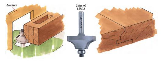
**4.** Use a piece of waste material behind the rail to prevent splintering. This is known as a 'spelch piece'. With the shoulders of the tenons complete, cut the profile on the stiles and rails. Once again, mount the profiler in the table with the bearing on the cutter slightly proud of the backfence to govern the depth.
