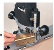
Hinge placed between depth stop and turret stop
