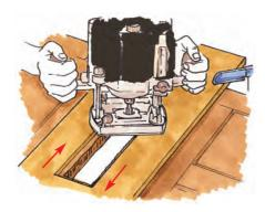
4. Rout in a clockwise direction around the aperture, taking several passes to complete the operation.
