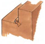
The seal is very versatile and can be routed into the apex of the rebate in the frame.
