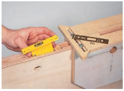
**3.** Clamp the jig to the door using a quick action clamp. A 32mm guide bush is used for mortise and a 26mm guide bush for the face plate. Rout in a clockwise direction around the aperture. Remove the rounded corners of the recess of the face plate with a chisel. Increase the depth of the mortise with a chisel or 3D-Bit<sup>®</sup> if the lock body is over 75mm in length.
