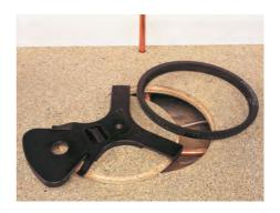
2. The router is fitted with a 30mm guide bush and the special cutter supplied with the jig. This cutter is designed specifically to suit the insert ring that is fitted later. Insert the router into the jig and rout in a clockwise direction in a series of passes until the cutter finally bottoms on its depth stop.
