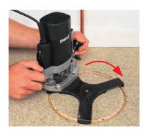
The Routabout system offers a unique solution found on site where access is required to pipes and electrical work beneath an 18mm or 22mm chipboard floor.
