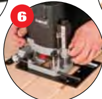
6 False Panel Groove Copier For creating repeated grooves.
