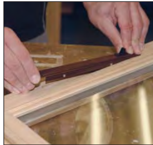
And fit both sides of the Trickle vent. The system produces a 12mm groove for a standard Trickle Vent.
