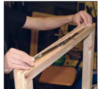
And fit the Espagnolette lock. The system caters for Espagnolette Locks 22mm, or 26mm deep, and 12mm width.
