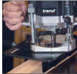
Rout the groove for the Espagnolette fittings with the jig (see page 57).
