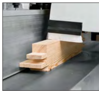
Profile all the components for the inner sash and outer frame profiles.
