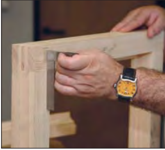
Dry assemble and check each joint.
