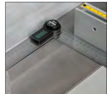
Ensure that the tenoning fence is set at 90 degrees to the back-fence.
