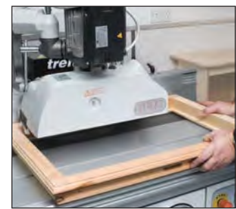
Once dry, using a spluch piece of timber run behind the sash to prevent break-out, machine the outside profile of each sash.
