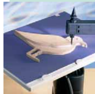
The parallel pin can also be used to follow two dimensional templates. Allow the pin to run lightly against the template edge to avoid any misalignment when changing direction.
