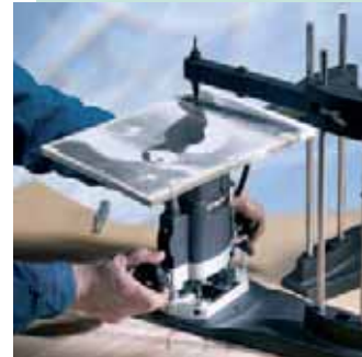
Start cutting by smoothly plunging the router to the cutting depth and following the line with the stylus.
