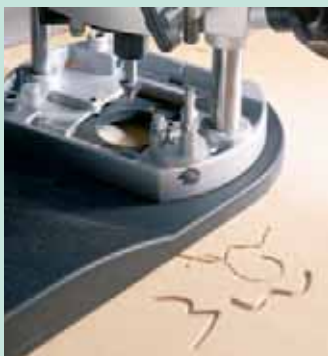
Set the cutter depth to give the required line strength.
