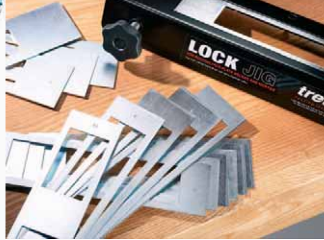
A range of templates to suit most popular makes of locks and latches are supplied with the Lock Jig.
