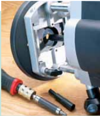
Centring the router stand baseplate using the guide bush and alignment pin provided.
