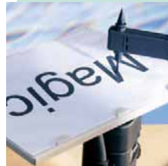
Signs, nameboards and logos can be reproduced, following a photocopy or computer print out. For these applications, use the parallel pin.
