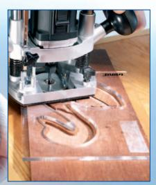
For template routing, a 16mm diameter guide bush is supplied with the T3 router. Other diameter guide bushes are available from the standard T rend range, allowing the T3 to be used with jigs such as the DJ300 dovetail jig.
