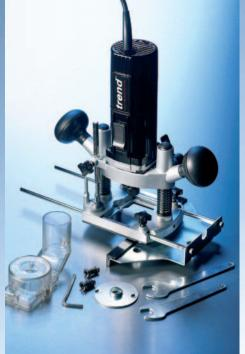
Accessories supplied with the T3 router include a side-fence, dust extraction adaptor, a 16mm guide bush and 2 extra collets, a 6.3mm collet fitted to router and 6mm and 8mm alternatives. A spindle/body lock spanner is included as well as the collet nut spanner.
