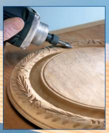
The body of the T3 router can be detached from the base unit to allow the T3 to be used as a hand-held carving or die grinding tool, using multi-flute burrs or grindstones. Do not use standard router cutters for these applications.
