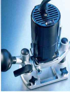
The smooth plunge action on the T3 can be locked at the required cutting depth using the positive action lever lock. The cutting speed can be pre-set between 8000 and 24000rpm using the step-less dial on top of the router body.
