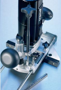
For fast repetitive applications, the T3 is fitted with a three-stage turret stop and graduated depth-gauge rod. The T3 will also accept optional accessories from the Trend T5 router range, such as the fine height adjuster.
