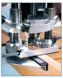
The Trend T3 router can be used for light duty routing applications, including edge moulding, rebating, trimming and template work. The standard TBC base configuration allows the T3 to be fitted to most Trend jigs and accessories.
