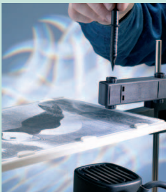
Adjust the table height to leave clearance above the routers cooling vents. Fit the O ring to the stylus and slide it into the copy arm.
