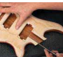
Making adjustments to the neck aperture.
