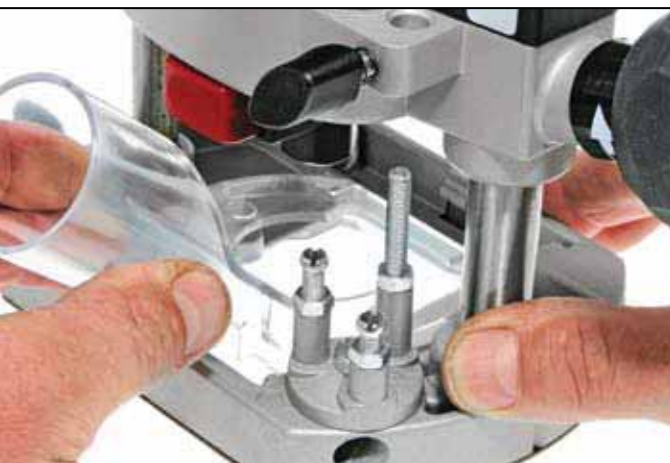
Fitting the new low profile dust spout.
