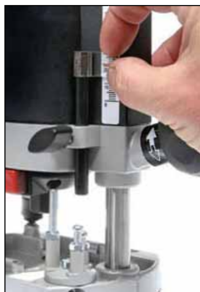
Adjusting the depth flag for depth of cut.
