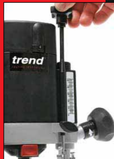
Adjusting the fine height adjuster.
