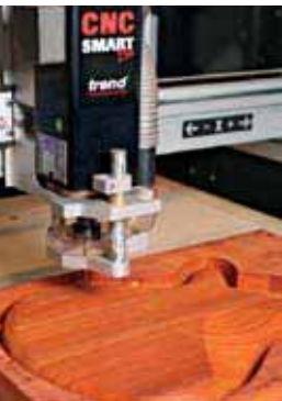
The CNC Smart cutting and then moulding the outside shape.
