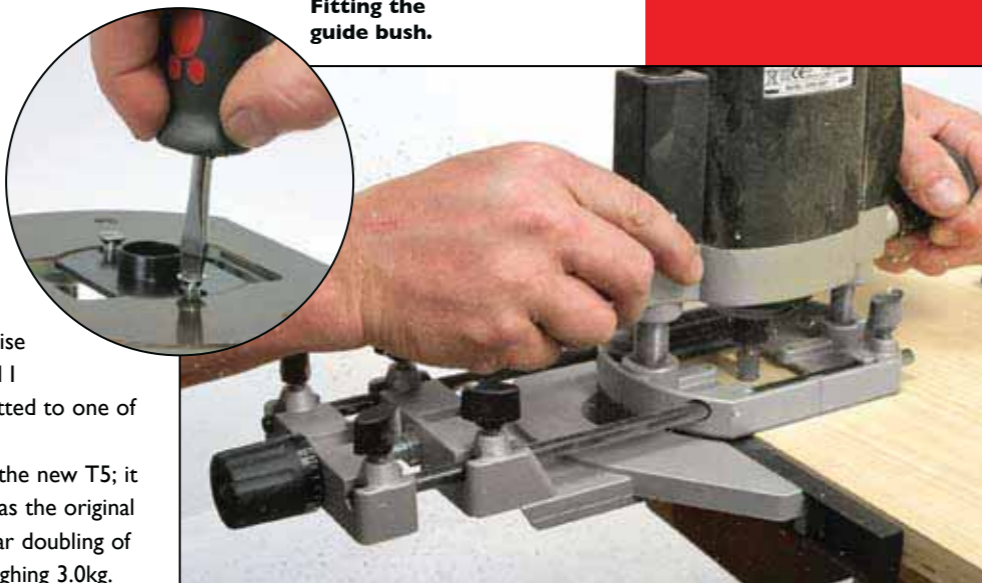
Micro adjustment side-fence.
