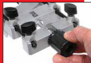
Adjusting the fence using the microfence adjuster.
