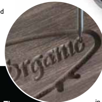
The Organic Guitar logo is machined out using a very small solid carbide spiral cutter before it is gold leafed.
