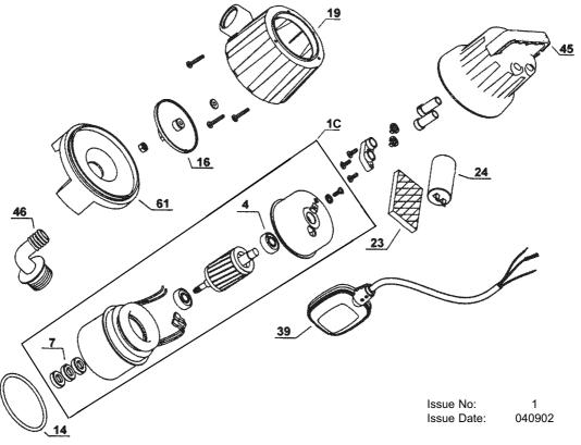
Item Part No. Description Item Part No. Description EL3001C EL10023 1C Complete Motor 23 Sponge 4 7 FI 10004 24 FI 10024 Bearing Capacitor 39 FI 10039 FI 10007 Oil Seal Switch 14 45 EL10045 Upper Body EL1014E O-ring 16 EL40016 46 EL10046 Impeller Connector EL20019 EL50061 Suction Base Pump Body
