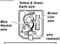
FUSE RATING THIS PRODUCT MUST BE FITTED WITH A: 13 Amp FUSE
