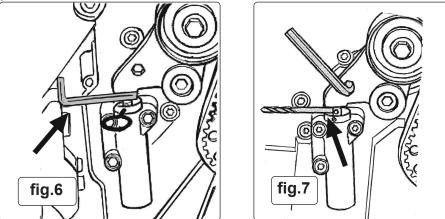
Remove the Hex Key and turn the hydraulic tensioner pulley arm anti-clockwise until the VS4593/1E Retaining Pin can be removed. Turn pulley arm back clockwise until a 7mm drill bit can be inserted between the hydraulic tensioner BODY and the tensioner pulley arm (fig. 7). Tighten the camshaft sprocket bolts and remove all tools.
