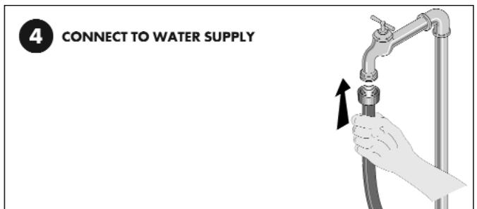
**4.2 Connecting the water supply.** Screw the hose connector to the water inlet on the machine (see fig.3). Use a reinforced hose pipe with an internal diameter of 1/2" and connect to the mains water supply as indicated in fig.4.
