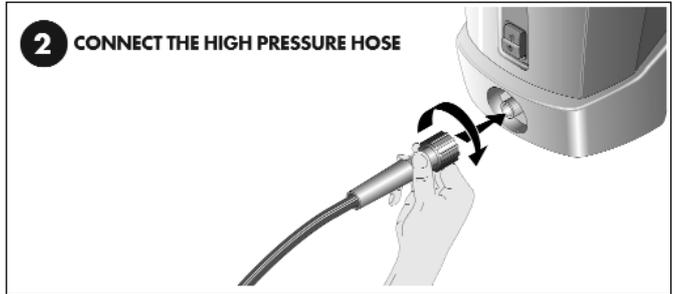
**4.1 Connecting the high pressure hose.** Remove and discard the transit plug from the water 'out' connector on the lower front of the machine (see fig.1). Attach the high pressure hose as indicated in fig.2 ensuring that the connector is tight.
