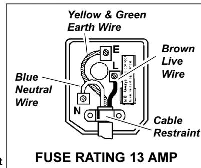
Double insulated products, which are always marked with this symbol
