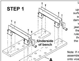
Lay the wooden worktop/jaws upside down on a surface that will not scratch or cause damage. Screw the vice arms to the jaws, ensuring that the jaw angle and ruler guides are on the same side as the vice handles at point "A"
