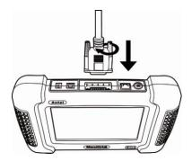
Figure 3.2: Main Cable Connection to the Scan Tool
