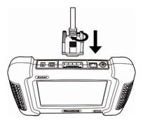
Figure 3.5: Main Cable Connection to the Scan Tool
