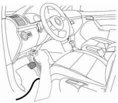
Figure 3.3: OBD II Cable Connection to Vehicle DLC
