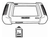
Figure 1.5: Memory Card into Scan Tool Slot
