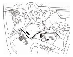
Figure 3.6: Main Cable Connection to Vehicle DLC
