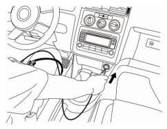
Figure 3.8: Plug into the Vehicle's Cigarette Lighter Receptacle
