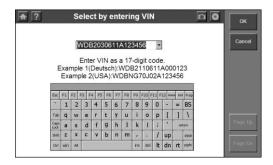
Figure 3.15: Manual VIN Acquisition Screen
